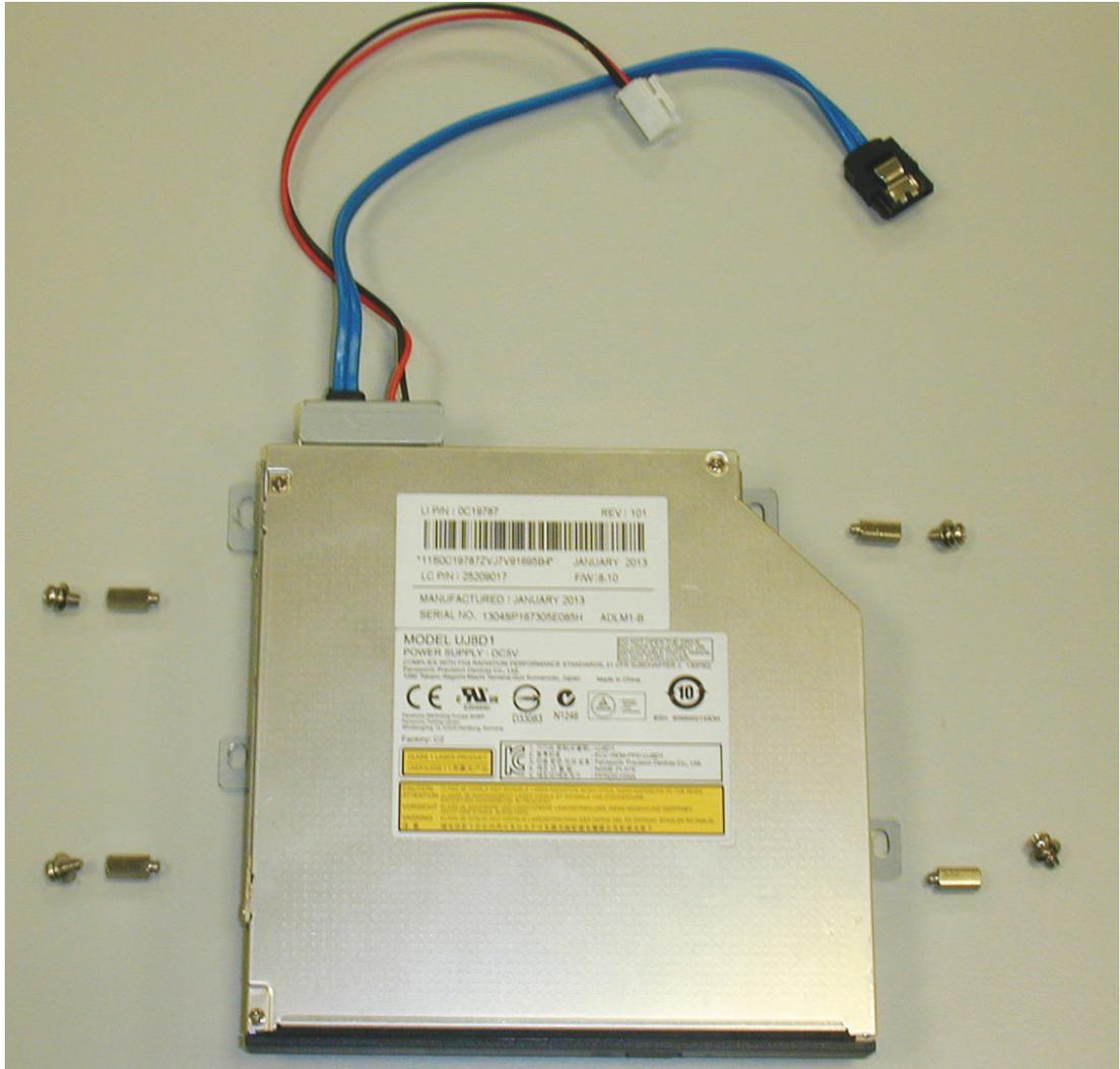
Figure 11.9: DVD install components for DIVAR AN 5000
