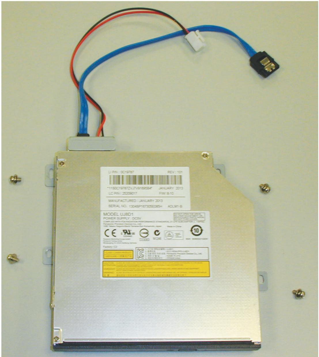
Figure 11.7: DVD install components for DIVAR AN 3000
